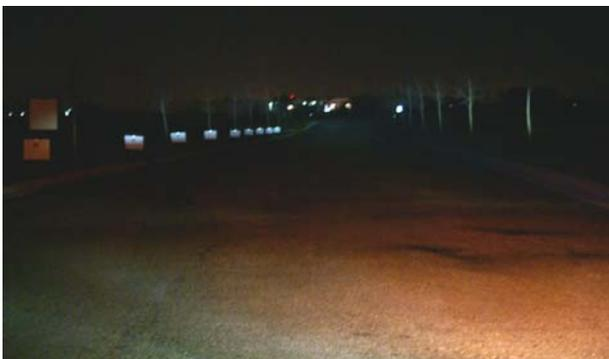
**bogie:** The shot to the left is of the high beam of the P7 only – covering up the low beam. Notice only the top edge of the distance markers are illuminated on the left; the upper portion of the trees on the right; almost no light on the street directly in front of the bike; but, the curbing and pavement are lit at and well beyond the 100 yard marker.
